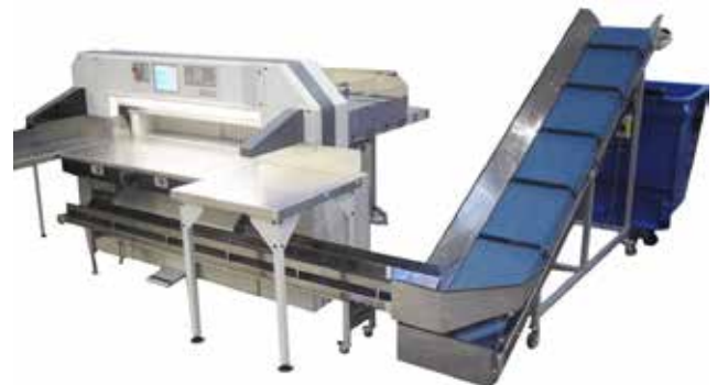
90°-deflection outside the area of the pneumatic table
