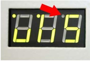
Right dot shows correct function of sensor of feeding table.
