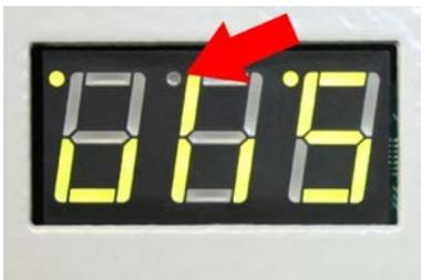
Middle dot shows correct function of sensor of counter.
