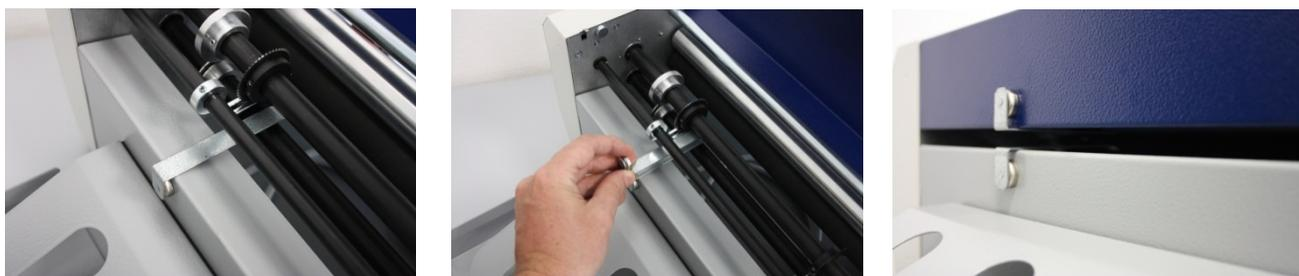
To remove the perforating wheels or the creasing wheel, it is necessary to remove the shaft with the strippers first and then remove the shaft with the perforating wheels. Remove the shaft by holding the bearing (39) and pull it over the spring into the terminal position. Then push the whole shaft back including the bearing that you continue to push into the terminal position, and remove the shaft from the machine as per the figure.
