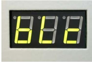
Symbol "blc" appears if rollers are blocked and the motor is overloaded.
