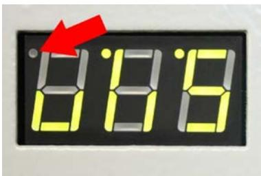
Left dot shows correct function of sensor, which defines revolutions of motor. Slowly move the pulley. If everything is ok, left dot stops shining always when sensor is not blocked by screen.
