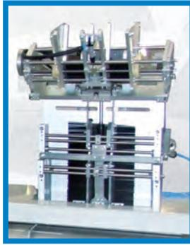
Hangers-forming and feeder for 100-300 mm. hangers.
