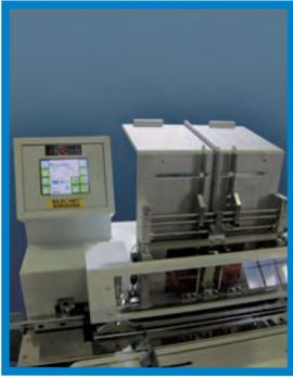
Touch-screen and hangers feeder for 100 a 300 mm.
